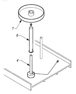
3-2. Attaching the Tension Release Set
