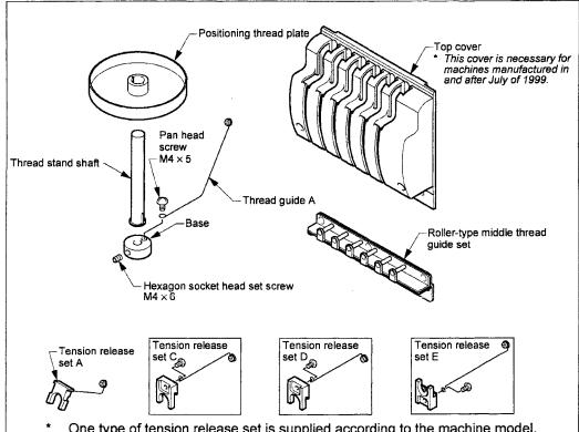
\* One type of tension release set is supplied according to the machine model. Applicable tension release type for the individual machine models is shown below.
