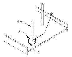
NOTE: Attach the base (2) in the direction so that the thread guide A (1) will not interfere with the adjacent thread cone. For example, the thread guide A (1) should be set in the rear right direction as shown below.
