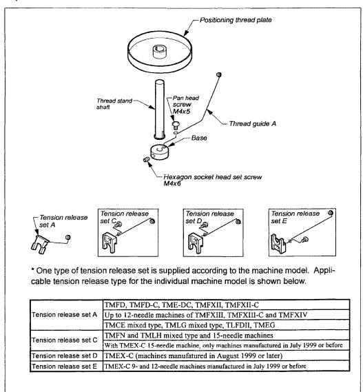
Page 4 Section 3-3 "Attaching the Roller-type Middle Thread Guide Set"
